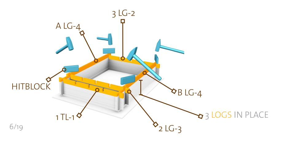
INSTALL THE FLOOR BEAMS AND ATTACH THEM WITH SCREWS.
