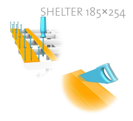
10 SCREWS INTO THE FIRST FLOORBOARD, 5 INTO EACH NEXT.
