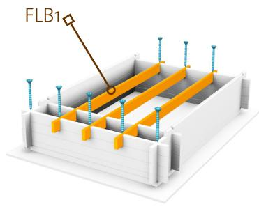
INSTALL THE FLOOR BEAMS AND ATTACH THEM WITH SCREWS.
